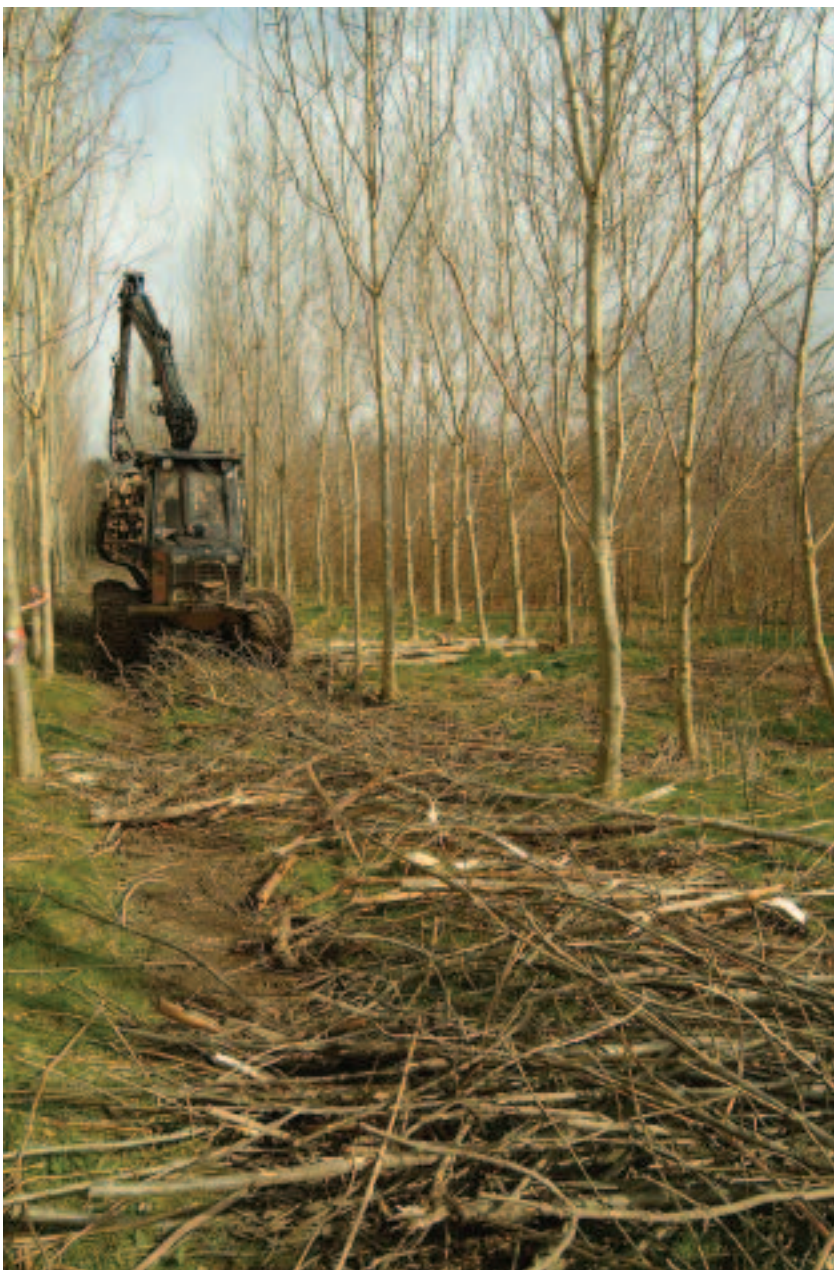
Forwarder taking thinning logs out of a ash stand. Note the brash mat.
