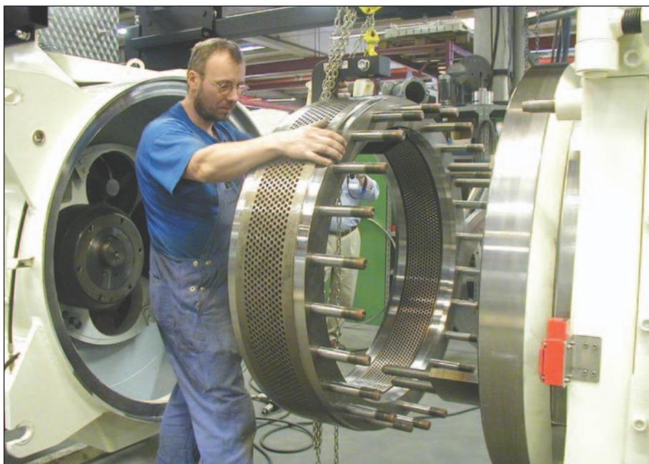
◀ Matrix being set up to press sawdust into pellets.
