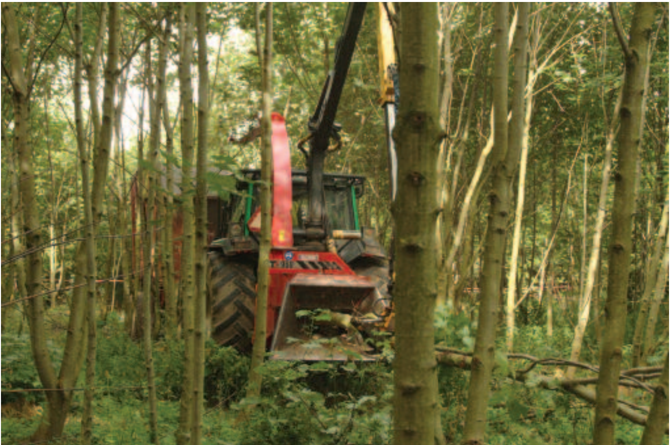
Tractor mounted TP 280 chipper on a Valmet tractor towing a high tipping trailer.
