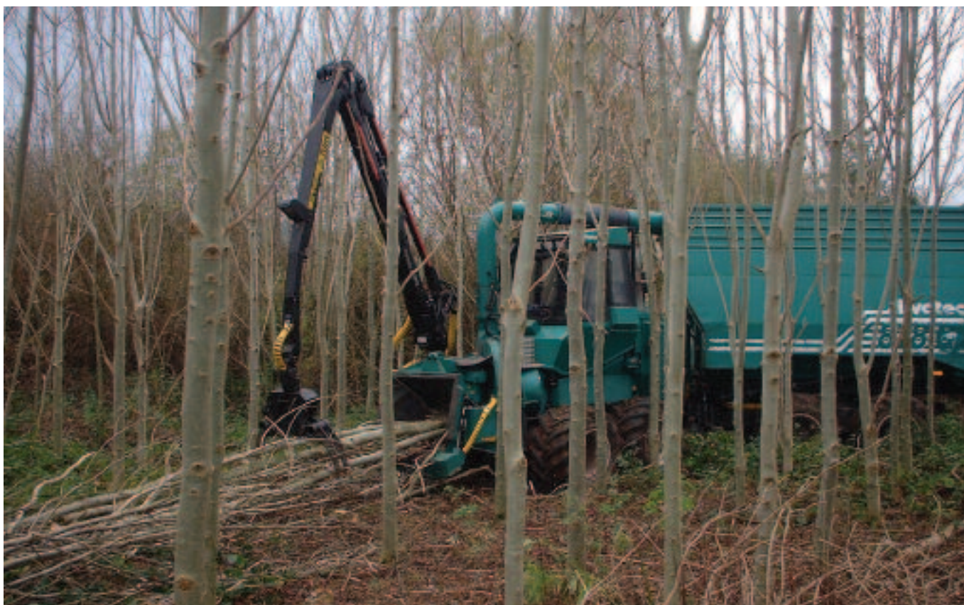
Silvatec chipper in an ash thinning. Note that in this case the trees are chipped from the top, which is not the preferred method.
