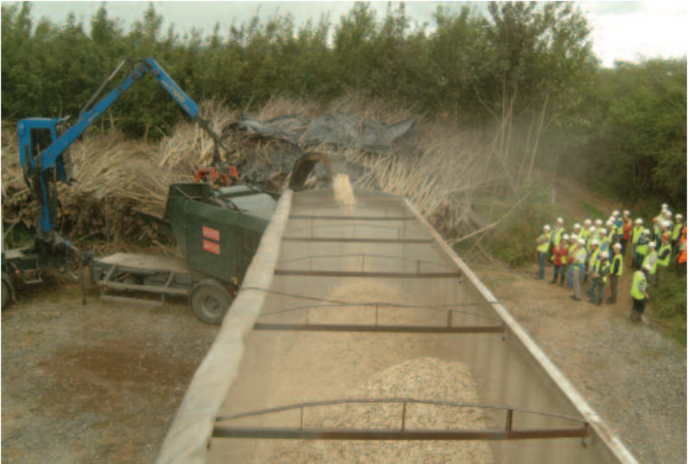
Jenz 700 truck mounted chipper blowing chips from the pile of whole trees into a walking-floor truck.
