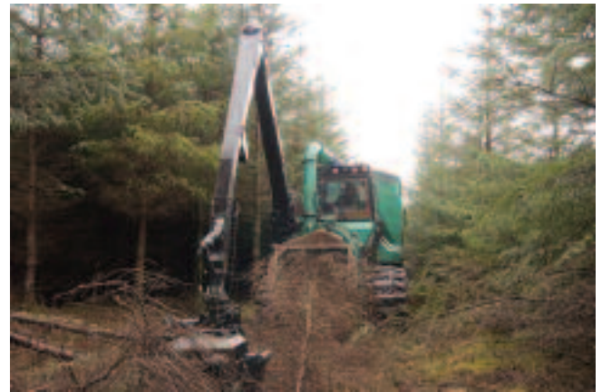
Chipping the line trees by Silvatec terrain chipper. Note the bandtracks on the wheels.
