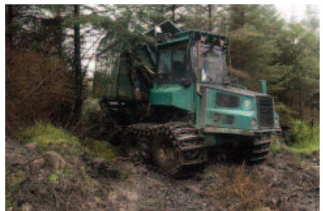
Chip forwarder coming to the road with a load of chips. Note the bandtracks.
