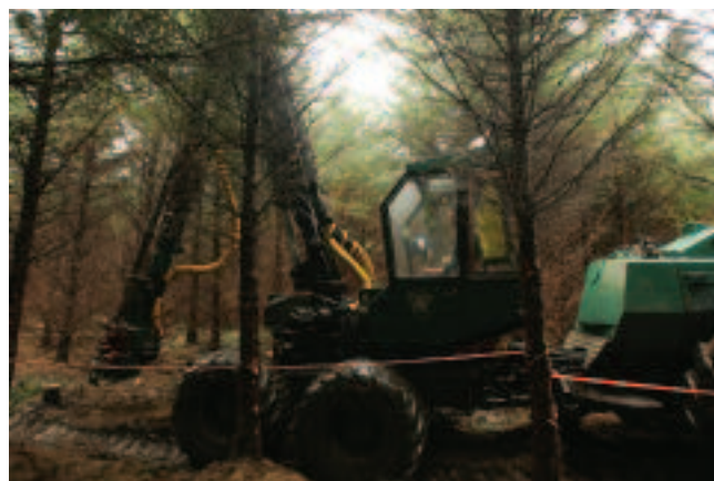
Silvatec feller-buncher in operation.
