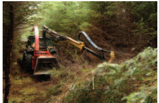
TP280 tractor-mounted front-fed chipper in line thinning. The trees are not yet completely dead.
