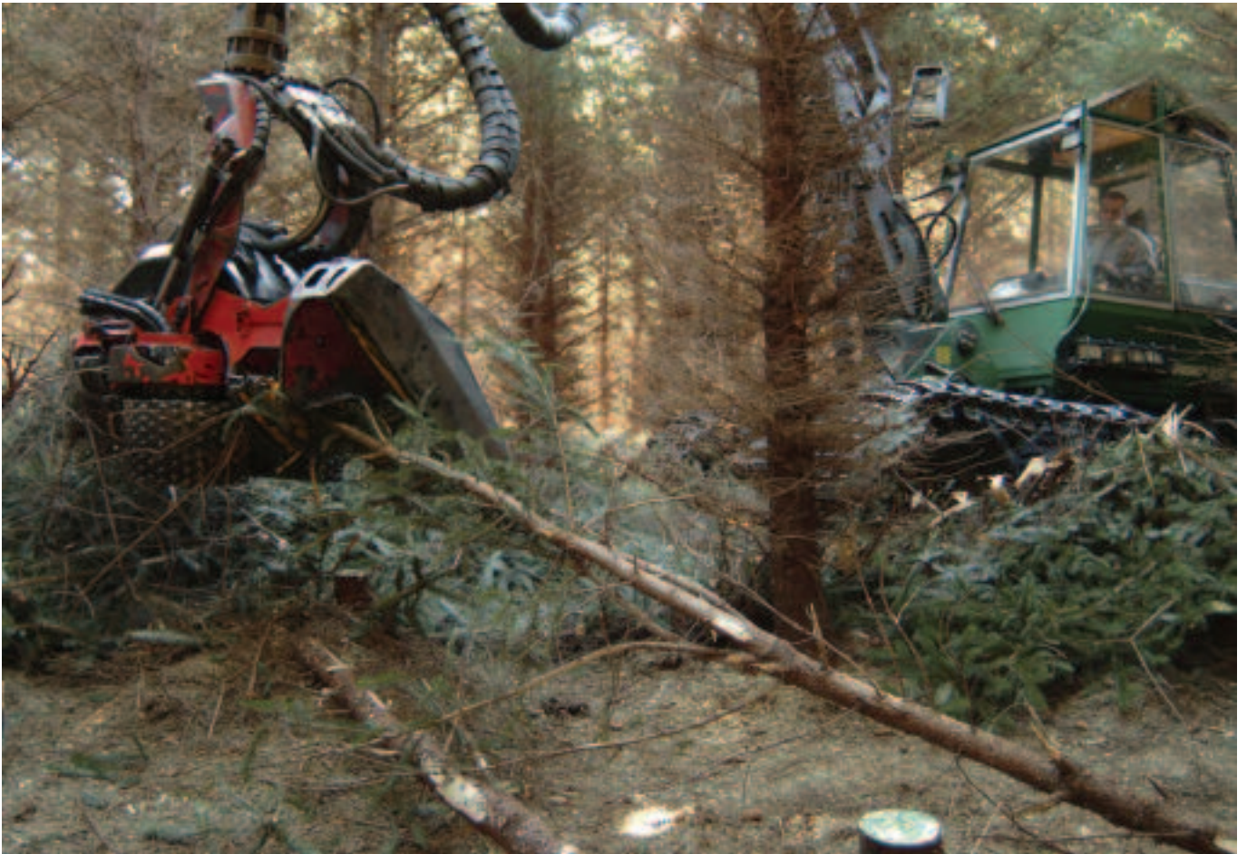
Harvesting energy wood, note crude delimiting and small top diameter.
