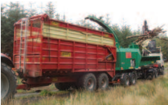
Jenz 700 truck chipper feeding into a tractor-trailer combination.
