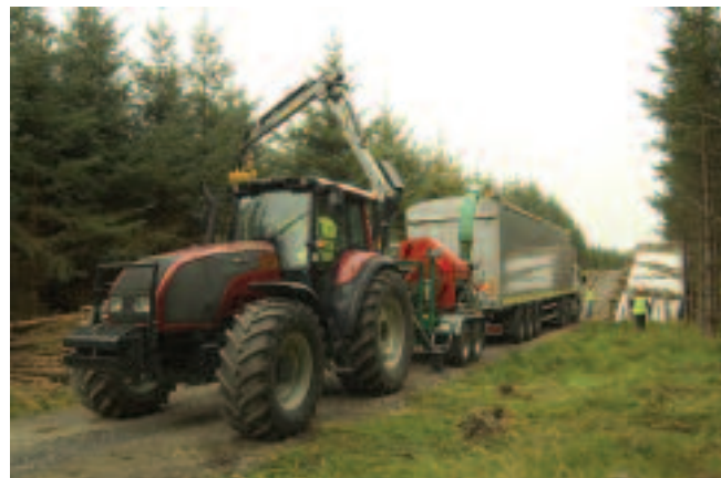
MusMax tractor-powered chipper blowing chips into a walking-floor truck.
