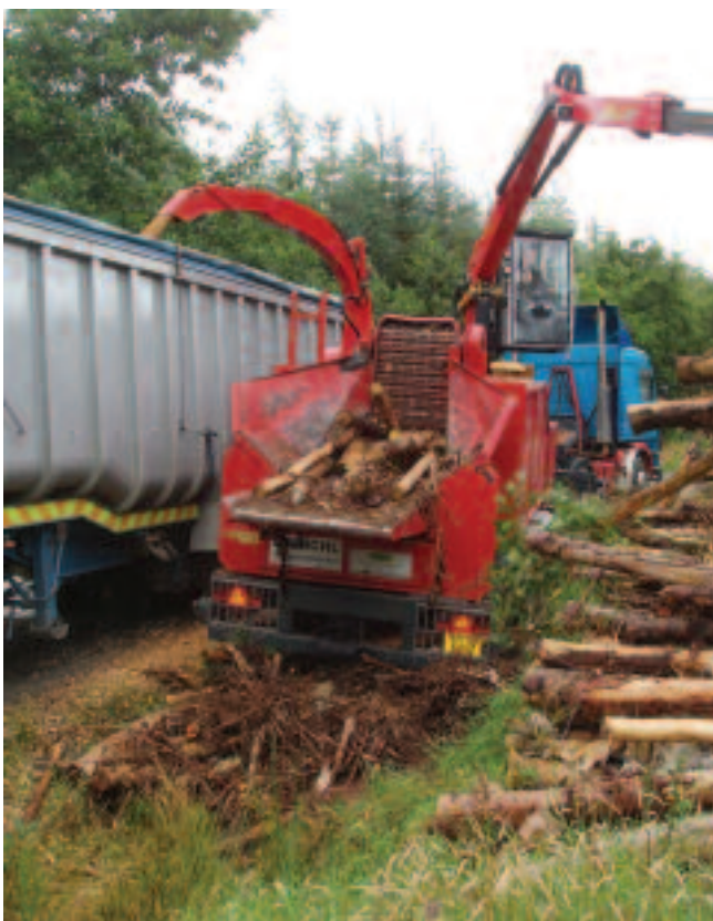
Starchl chipper blowing chips into truck.
