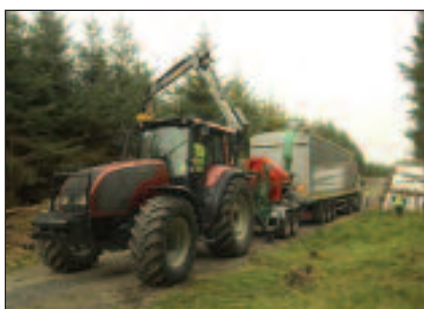
MusMax tractor-powered chipper blowing chips into a walking floor truck.
