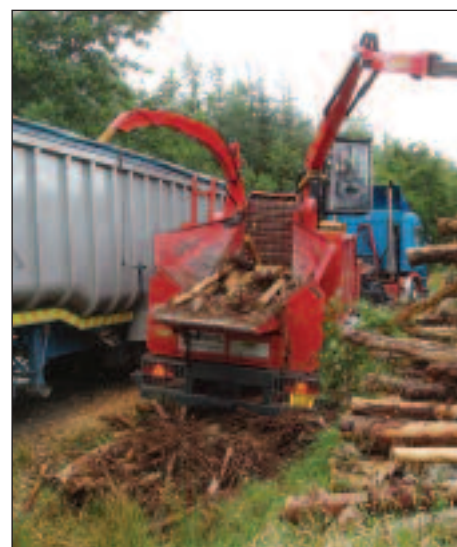
Starchl chipper blowing chips into truck.
