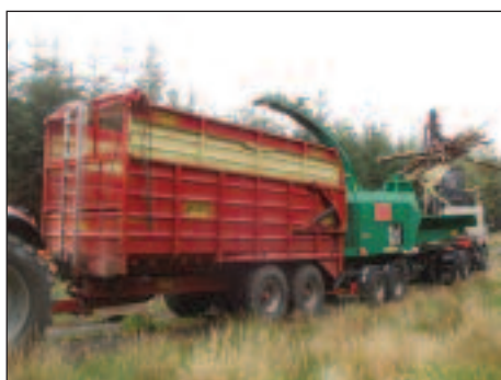
Jenz 700 truck chipper feeding into a tractor-trailer combination.
