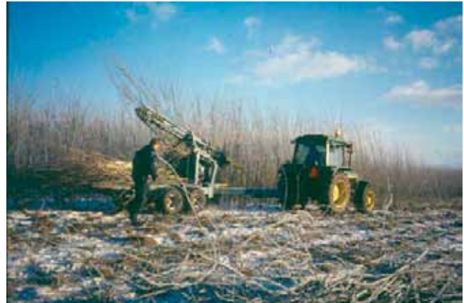
Figure 1: Frobesta whole-shoot harvester drawn by tractor.
