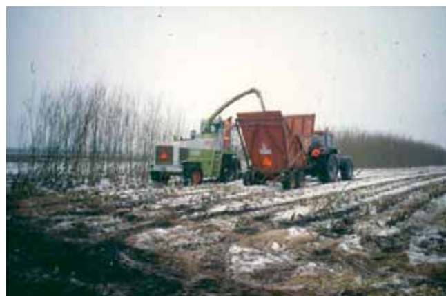
Figure 3: A Claas silage harvester blowing chips into a tractor trailer unit.
