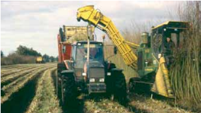
Figure 4: Austoft self propelled harvester unloading into tractor-trailer combination.
